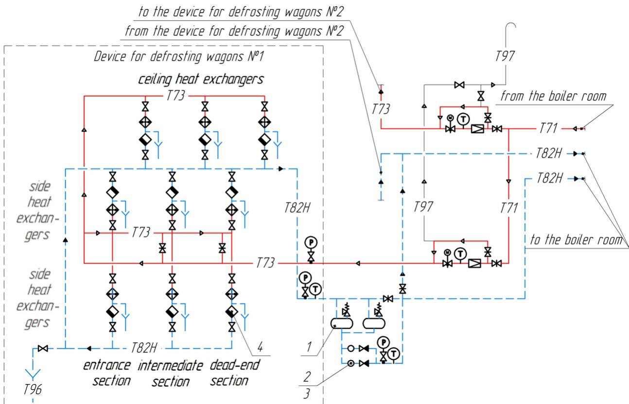
Fig.7. Basic energy diagram of the modernized steam supply system of technological defrosting houses (modernization positions: 1 – condensate collecting tank, 0.005 MPa; 2 – Ks-12-50 condensate transfer pump; 3 – device for frequency regulation of the Ks-12-50 Danfoss VLT 2800 A3 pump drive, 4 – Spirax Sarco FT14HC steam trap). Other designations correspond to the designations given in Fig. 2)
