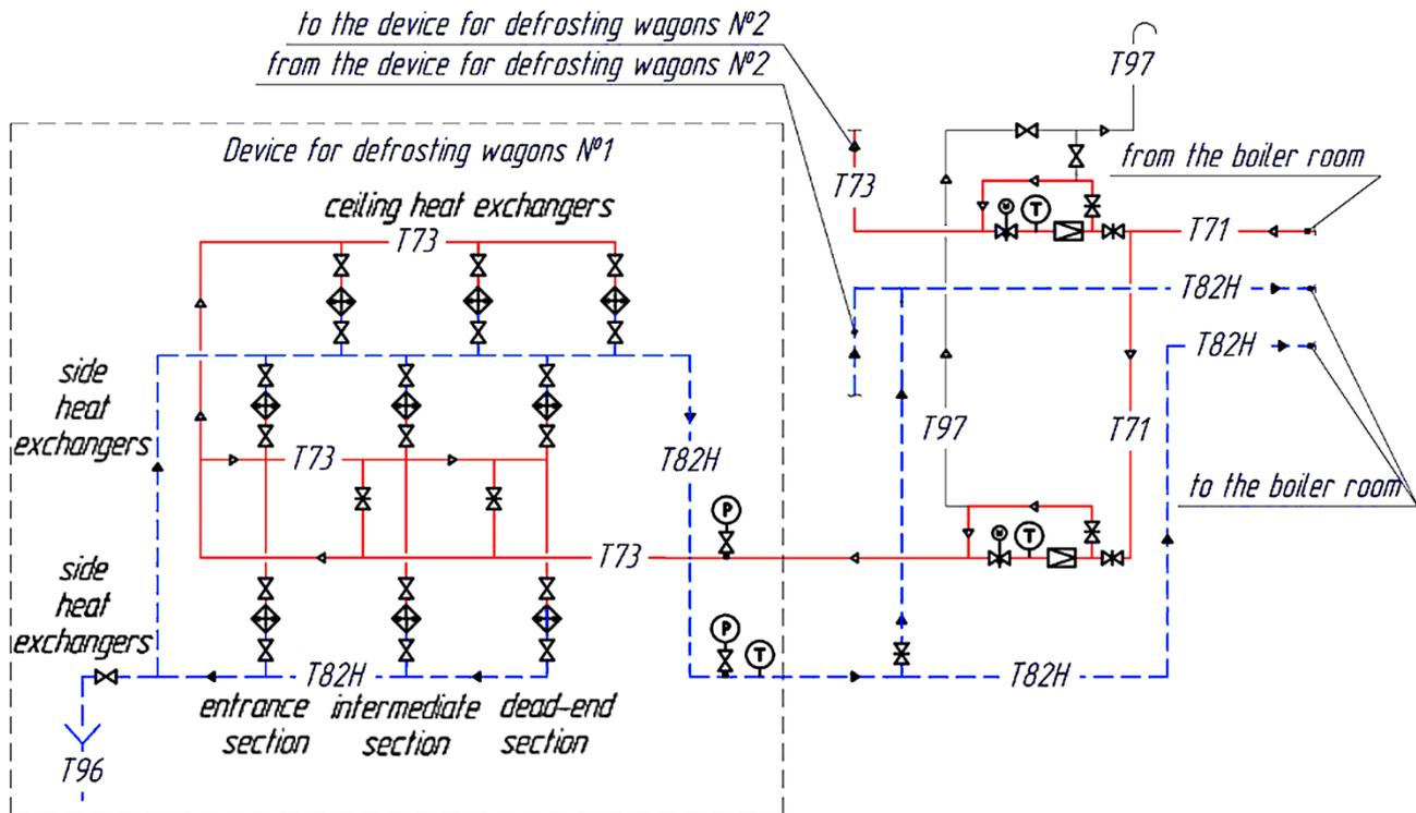
Fig. 2. Basic energy scheme of the existing steam supply system of process defrosting houses (T71 – pipeline of superheated water vapor ( $P^*=0.8$  MPa,  $T=200...220$  °C); T73 – pipeline of moist saturated steam after reduction ( $P=0, 2...0.3$  MPa); T82N – supercooled condensate pipeline ( $P=0.18...0.25$  MPa,  $T=102...106$  °C); T96 – drainage pipeline; T97 – pipeline for blowing ; (notations according to SSTU B A.2.4-8:2009; \*- the amount of excess pressure is given)
