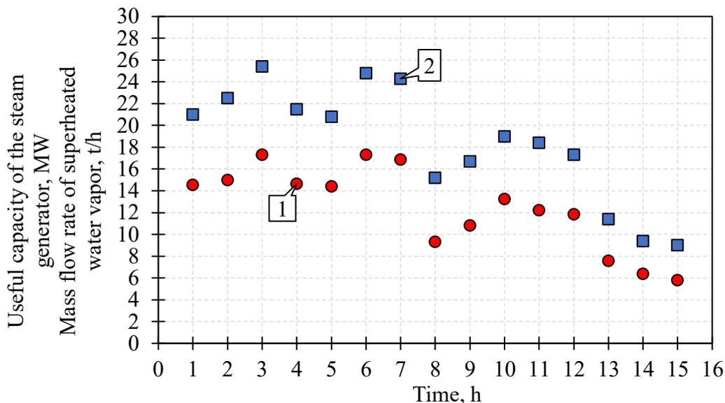
Fig. 4. Dynamics of changes in the useful thermal power of the object  $Q_{SV}$  and consumption of superheated water vapor  $D_{SV}$  at the time of measurements, 1 – useful thermal power; 2 – consumption of superheated water vapour
